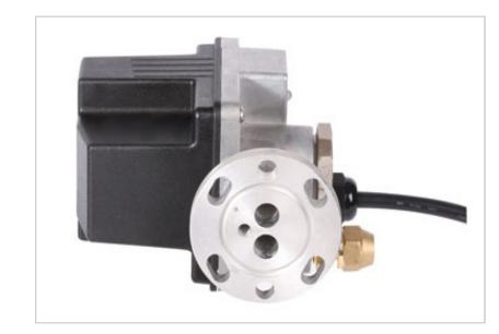
OUT280 monitors and controls the oil level in the refrigerant compressors. In particular, the problem of bad oil distribution in multi-compressor packs is solved, thanks to active oil supply from a shared oil reservoir. The oil level regulator keeps the oil level between 40% to 60% height of the sight glass.
