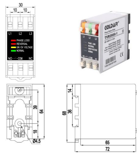
Insert the relay into 35mmTH Rail mounting directly. Under other installation, use M2-M4 type screw to fix.
