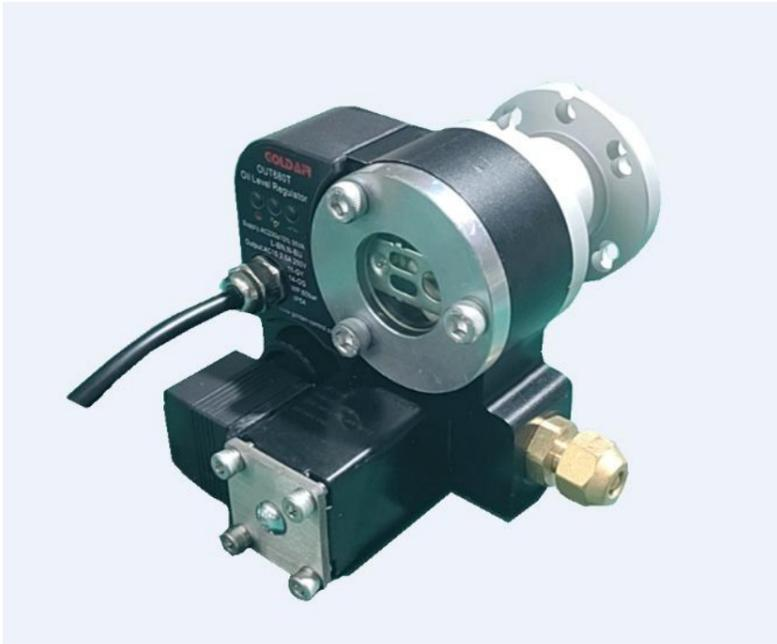
OUT680 monitors and controls the oil level in the refrigerant compressors. In particular, the problem of bad oil distribution in multi-compressor packs is solved, thanks to active oil supply from a shared oil reservoir. The oil level regulator keeps the oil level between 40% to 60% height of the sight glass.
