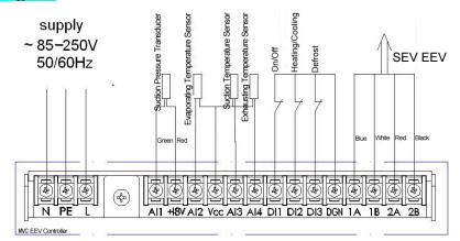
Heating/Cooling: On for heating; Off for cooling. On/Off: From Off to On, means On signal; Opposite, means Off signal. Defrost:From off to On, means on Defrost; Opposite, means exit from Defrost state.
