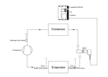
Model specification: evaporating temperature: -50~-15°C
