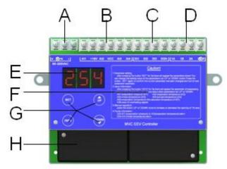
A. The input connection of the power of the controller: the power when the controller works normally is  $85\sim260$ VAC 50/60Hz.
