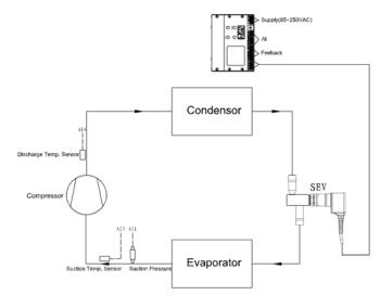
Model specification: the evaporation temperature:  $0 \sim 15^{\circ}$ C Wind-cool heat pump cold and hot water unit, wind-cool heat pump direct evaporation unit. (The flow in the picture is the work condition of the refrigeration)
