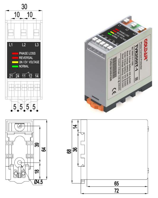
Insert the relay into 35mmTH Rail mounting directly. Under other installation, use M2-M4 type screw to fix.
