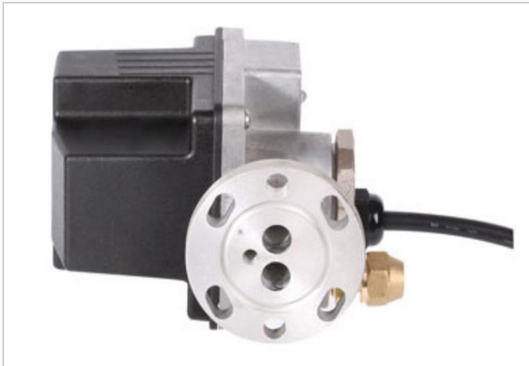
OUT280-II monitors and controls the oil level in the refrigerant compressors. In particular, the problem of bad oil distribution in multi-compressor packs is solved, thanks to active oil supply from a shared oil reservoir. The oil level regulator keeps the oil level between 40% to 60% height of the sight glass.
