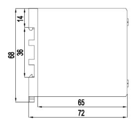
Insert the relay into 35mmTH Rail mounting directly. Under other installation, use M2-M4 type screw to fix.
